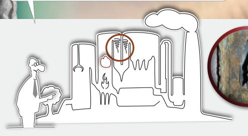
During the combustion stage, fly ash is generated which, dragged by the warm gas current and given its rather plastic and semi-molten state, clings to the walls of the furnace covering the top of the post-combustion chamber and the steam generator pipes.
