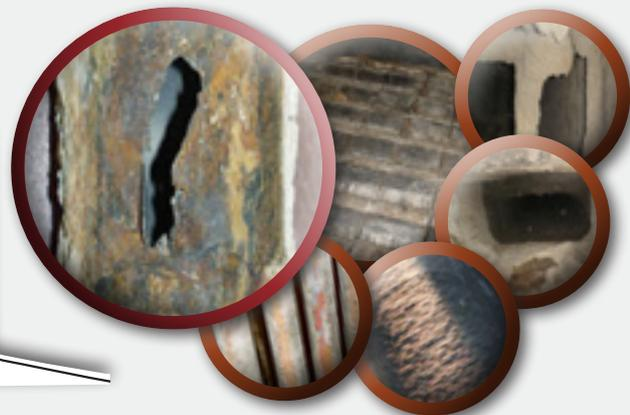
During the combustion stage, **fly ash is generated** which, dragged by the warm gas current and given its rather plastic and semi-molten state, clings to the walls of the furnace covering the top of the post-combustion chamber and the steam generator pipes.
